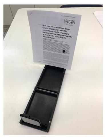
A full sheet of paper is held in place with fully extended stand back and magnet. Phone is positioned optimally from document.
